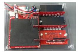
8) Attach the backplane to the plugs on both the cue strips and the vertical adapter board.
