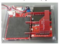
9) Re-assemble the module by placing the enclosure halves back together. Make sure no wires fit underneath the battery compartment.
