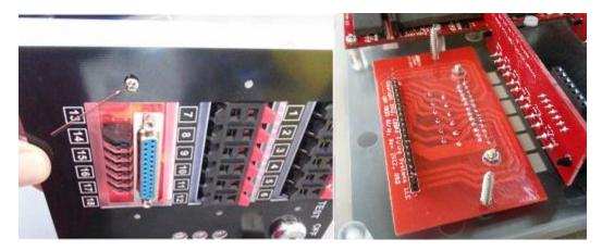
6) Attach the included plastic standoff to the other side of the screws. Repeat for both sides.
