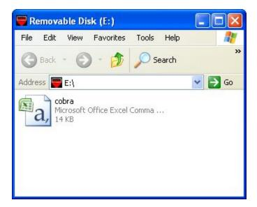
You are now ready to upload the script file into the COBRA 18R2. To perform this, simply plug the USB flash drive into the COBRA 18R2. If there are no errors, then the 18-cue LED grid will display all green. If there are errors in your file, the 18-cue LED grid will display all red and the error code(s) / line number will display / rotate on the script timing display.
