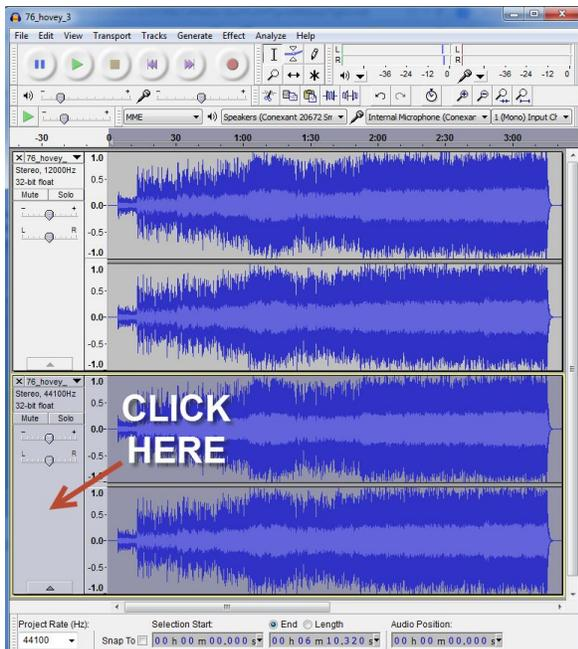
6. As shown above, click on the 2nd audio instance to highlight it. Then, click Edit > Remove Audio or Labels > Cut. This will remove the audio from the 2nd instance.
