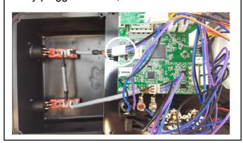
**Step 10)** Connect the 6" XLR cable into the J5 connector on the Audio Box board.
