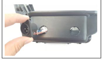
**Step 6)** Use drill to insert screws into top left and bottom right of each XLR connector.
