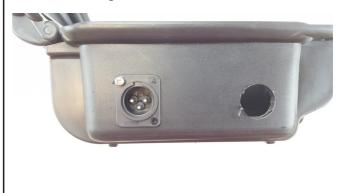
**Step 7)** Connect cables to XLR connectors as shown below.
