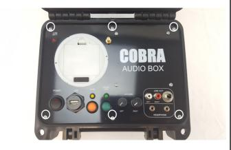
Step 2) On the left side of the armored case, measure and mark 1 3/8" from the left and right side of the case.
