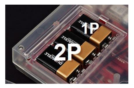
**Important!** COBRA recommends using higher quality battery brands such as Duracell or Energizer. If you plan to use re-chargeable batteries, we don't suggest using them for the 2P firing cue batteries, only the 1P battery. Make sure your battery is at least 500mAh in order to maintain the published battery life specifications noted above.
