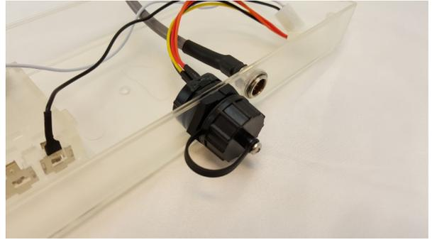
**Step 5)** Plug the battery harness and USB port harness back into 18R2.
