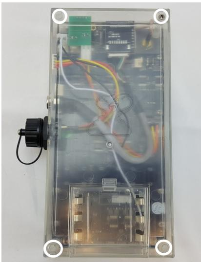
**Step 8)** Insert the Deadman trigger into the Deadman port, button side up. You're now finished installing your Deadman!
