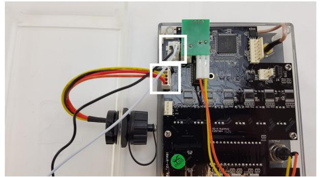
**Step 3)** Unscrew the USB cap and nut. Then push the USB port inward to remove it from the 18R2 back enclosure.
