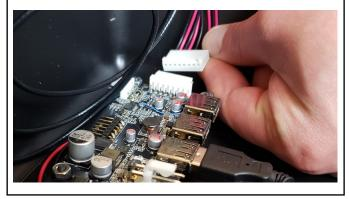
**Step 21:** Connect the Command Center keyswitch harness to CN7 on the Power board.
