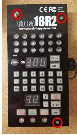
**Step 3:** Disconnect the keyswitch harness from the remote, unscrew the keyswitch nut to remove the keyswitch.
