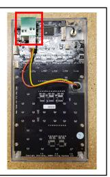
**Step 8:** Set the remote enclosure in place underneath the Command Center faceplate, and fasten the remote mounting screws in the four corner holes.
