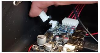
Step 22: Connect the Deadman harness (If installed on 18R2) and SMPTE harness.
