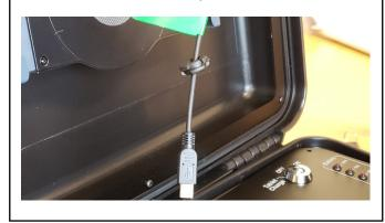
**Step 19:** Connect the micro USB end of the tablet OTG/Charge harness (Green) to CN7 ("Tablet") on the OTG board.
