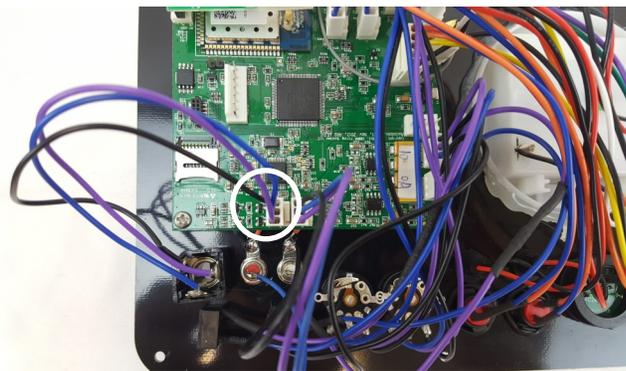
**Step 9)** Connect the cable that was previously plugged into J5, into male XLR cable.
