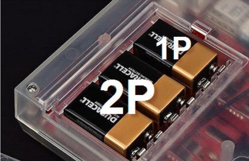
**Important!** COBRA recommends using higher quality battery brands such as Duracell or Energizer. If you plan to use re-chargeable batteries, we don't suggest using them for the 2P firing cue batteries, only the 1P battery. Make sure your battery is at least 500mAh in order to maintain the published battery life specifications noted above.
