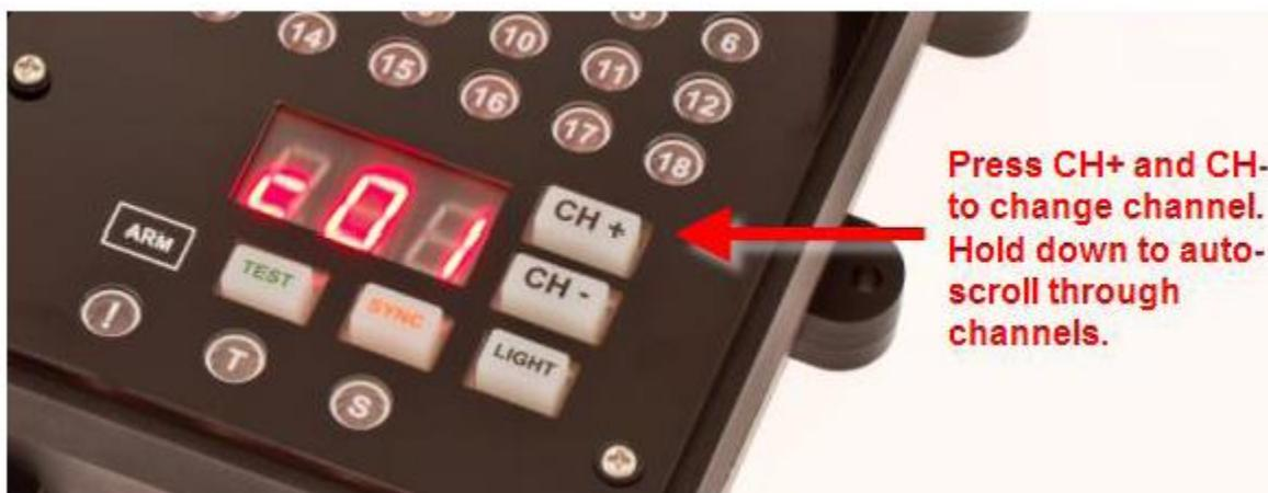
Press CH+ and CH- to change channel. Hold down to auto-scroll through channels.
